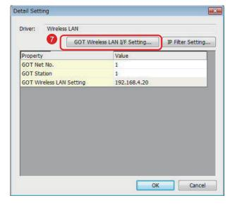
Set the IP address of the wireless LAN communication unit. Click [GOT Wireless LAN I/F Setting].
