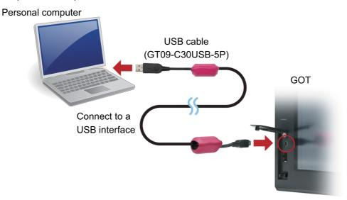
Open the front cover and connect the cable to the USB interface.
