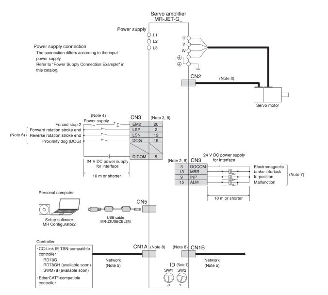
Notes: 1. The node address or the 4th octet of the IP address can be set to between 1 and 254 with a combination of the ID setting switches or the rotary switches (SW1 and SW2). Note that the number of the connectable slaves depends on the controller specifications.
