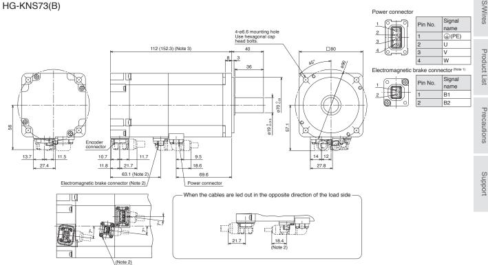
Notes: 1. The electromagnetic brake terminals (B1, B2) do not have polarity.
