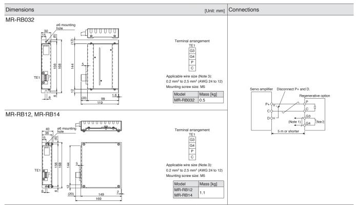
Notes: 1. Create a sequence circuit that turns off the magnetic contactor when abnormal overheating occurs.
