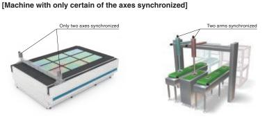
The two arms can avoid interference by synchronizing with each other, shortening the cycle time.
