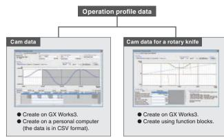
The operation profile data is divided into the following two types of cam data.
