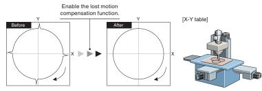
Suppression of quadrant protrusion of circular path
