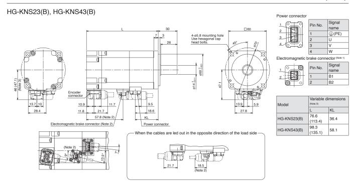
Notes: 1. The electromagnetic brake terminals (B1, B2) do not have polarity.
