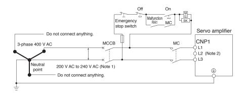
Notes: 1. Use a step-down transformer as necessary to keep the power supply voltage between 200 V AC and 240 V AC. 2. For 1-phase 200 V AC to 240 V AC, connect the power supply to L1 and L3 terminals. Do not connect anything to L2.
