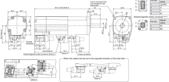
Notes: 1. The electromagnetic brake terminals (B1, B2) do not have polarity. 2. Only for the models with an electromagnetic brake.
