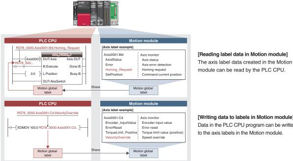
[Writing data to labels in Motion module] Data in the PLC CPU program can be written to the axis labels in the Motion module.
