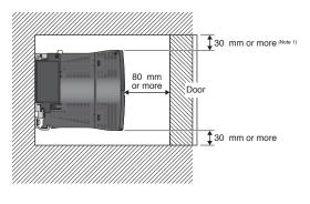
Notes: 1. Provide clearance of 30 mm or more when the height of a wiring duct is 50 mm or less. In other cases, provide clearance of 40 mm or more. 2. Provide clearance of 20 mm or more when an extension cable is connected/removed without removing a power supply module.
