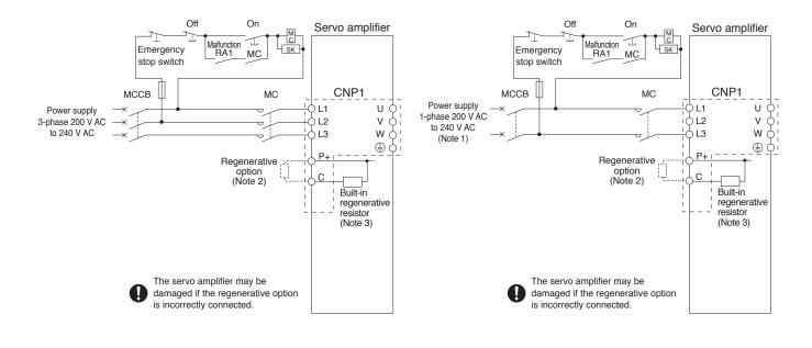
Notes: 1. For 1-phase 200 V AC to 240 V AC, connect the power supply to L1 and L3 terminals. Do not connect anything to L2.
