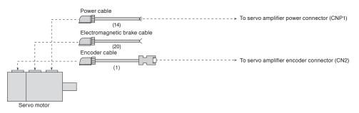
•For leading the cables out in the opposite direction of the load side (Note 1)
