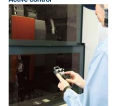
Adjusts the processing condition by a dial while looking at the processing.
