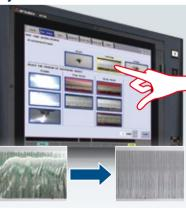
High quality processing regardless of proficiency is possible by selecting the similar picture to processing status.
