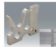
Material/Thickness Stainless steel (SUS304)/t10mm \*When using f254mm(f10") lens (option)
