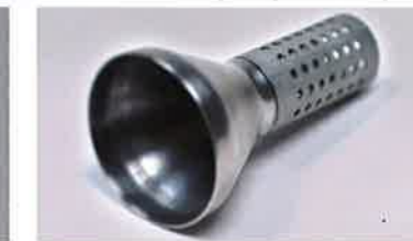
Stainless tube, thickness: t2.0mm Coated tube, thickness: t2.0mm Butt weld (assist gas: argon)
