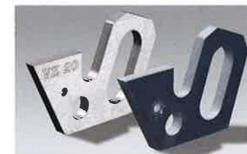
Left: t8.0mm stainless (assist gas: nitrogen) Right: t8.0mm aluminum alloy (assist gas: air)
