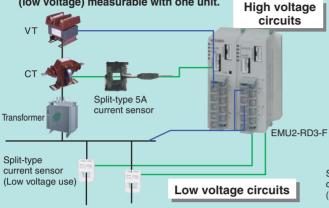
When measuring high-voltage circuits, use Split-type 5A current sensor (EMU2-CT5) in combination with VT and CT. At this time, pass the secondary side of the CT through the splittype 5A current sensor.
