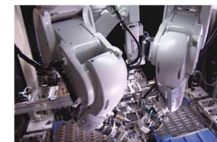
Assembly work that maintains the relative positions for mutual gripping
